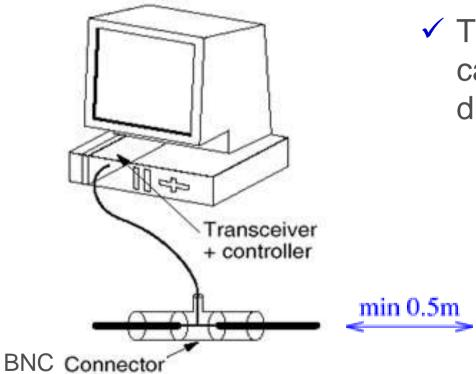
✓ Thinnet, simple coaxial cable, BNC connectors directly to the hosts
